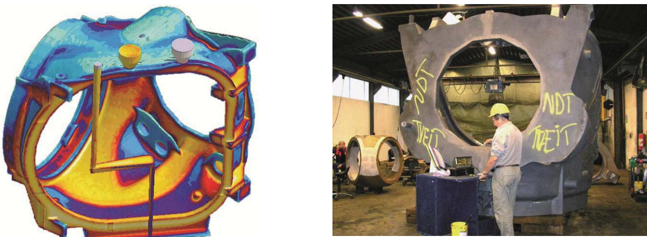
Figure 21: Casting process simulation strongly supports the development of wind power casting technology. Compared to welded parts, castings offer much better fatigue properties, which is essential for components with a required minimum lifetime of 20 years. The weight of the castings is a critical factor for the functionality and price of a wind turbine. This means designer and foundry must strongly cooperate to take full advantage of the material performance for an optimized part. /12/.
