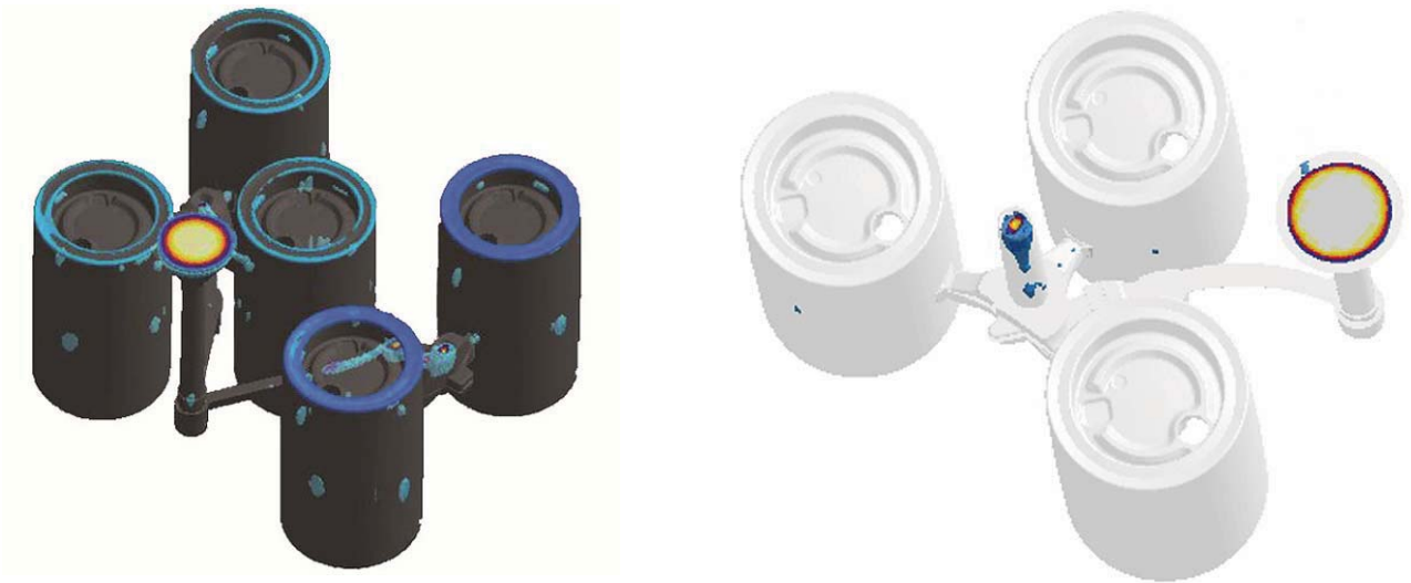
Figure 7: Is a riser needed or not? The porosity prediction for an original riserless lay-out for a grey iron grade 250 casting shows problems near the top surface (left picture). The simulation clearly demonstrates the liquid shrinkage to be the root cause of the problem. Porosity prediction for a modified layout shows that a small riser completely compensates liquid shrinkage (right picture) /8/.
